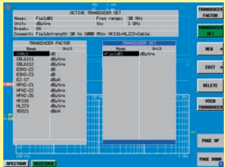
FIG 3 Frequency-dependent correction values with up to 50 reference values per data record (antenna transducer, cable attenuation etc) can be simply and easily generated and saved as a TRANSDUCER FACTOR. In addition, several transducer factors can be combined to form a TRANSDUCER SET. An automatic compatibility check ensures that settings are error-free. The number of transducer factors and sets which can be saved is practically unlimited. A variety of factors have already been programmed in the factory. With VIEW TRANSDUCER, every saved factor can be graphically displayed on the screen as a trace.
