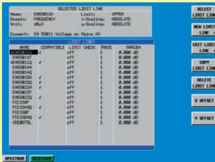
FIG 2 The ESPI supports the convenient generation and saving of practically any number of limit lines, with up to 50 reference points per line. Each limit line can have a fixed relation to one of three traces. Furthermore, a margin for a limit line (MARGIN) can be predefined and monitored (LIMIT CHECK). The limit values of the most important commercial standards have already been programmed in the ESPI.
