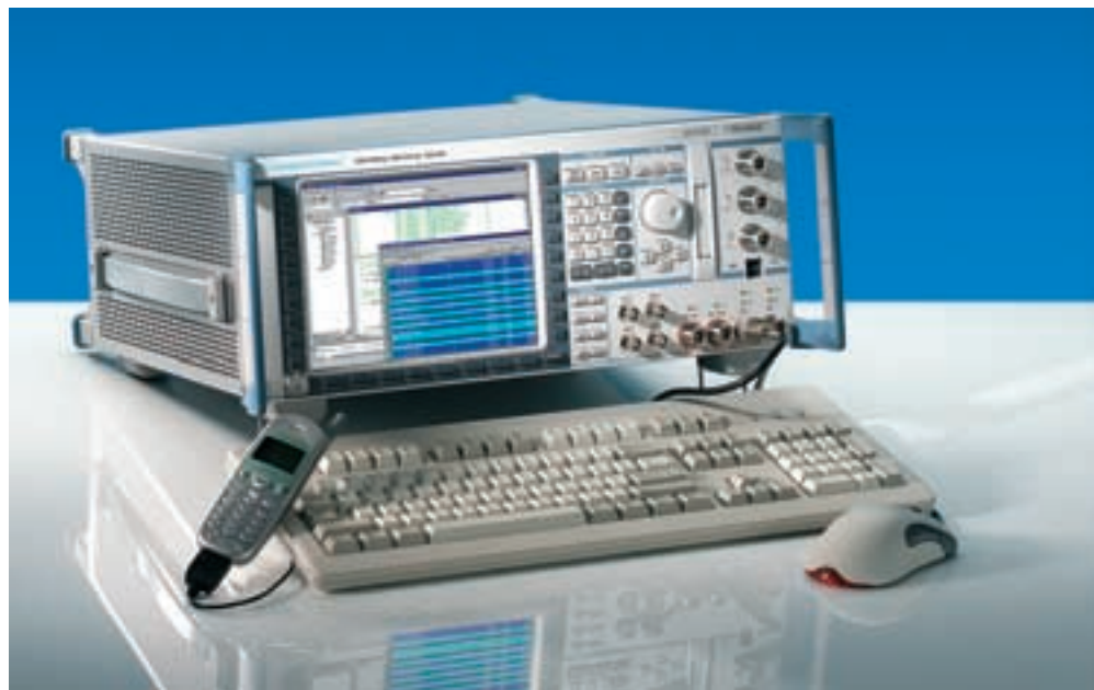
FIG 1 The Universal protocol Tester CRTU-G simulates a GSM base station where mobile phones can be tested with any imaginable signalling scenario
