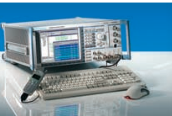
The GSM Protocol Analyzer CRTU-G simulates a GSM base station where mobile phones can be tested with any imaginable signalling scenario.
